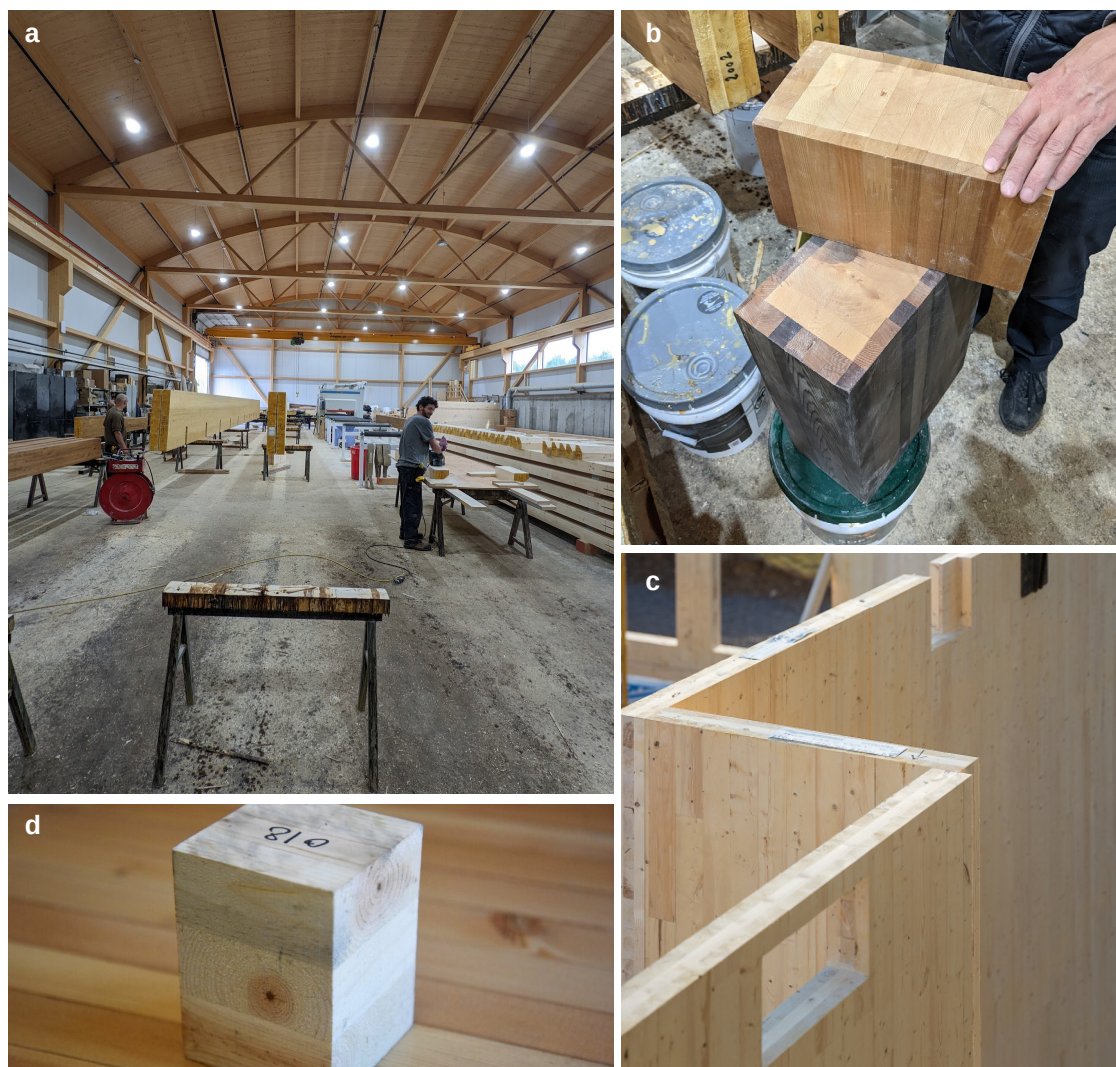
Fig. 4. a) Mass timber manufacturing facility near the study region (Art Massif, Saint-Jean-Port-Joli, Quebec) and b) test samples of a mixed hardwood veneer and glulam beam (photos: Osborne et al. (48)). c) Sample of a custom CLT panel utilizing low-value ponderosa pine (38). Popular industry CLT panel manufactured with black spruce (90% by volume) and other common building spies (spruce, pine, and fir; typically known as SPF).
